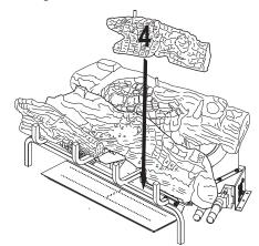
Figure 25 - Installing Log # 4
