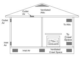
Figure 3 - Ventilation Air from Outdoors
