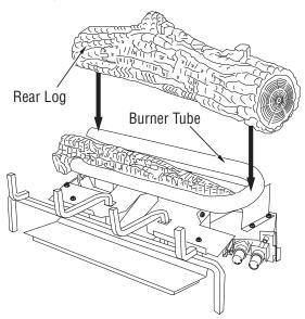
Figure 35 - Installing Rear Log
