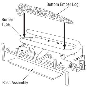
Figure 34 - Installing Bottom Ember Log
