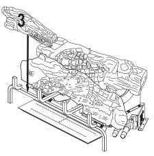
Figure 24 - Installing Log # 3
