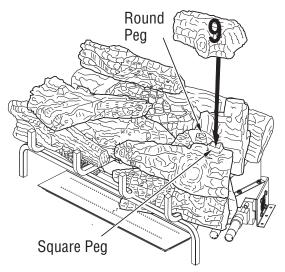
Figure 30 - Installing Log # 9
