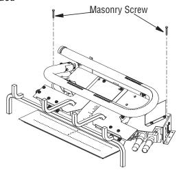
Figure 11 - Attaching Base to Fireplace Floor
