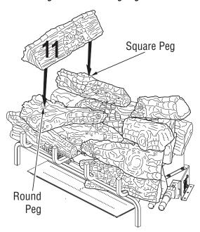
Figure 32 - Installing Log # 11
