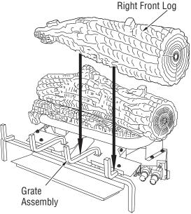
Figure 36 - Installing Right Front Log
