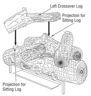
Figure 39 - Installing Left Crossover Log
