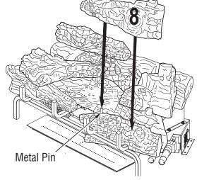
Figure 29 - Installing Log # 8
