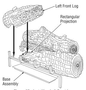
Figure 37 - Installing Left Front Log
