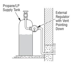
Figure 12 - External Regulator With Vent Pointing Down
