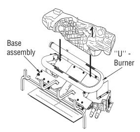
Figure 22 - Installing Log # 1
