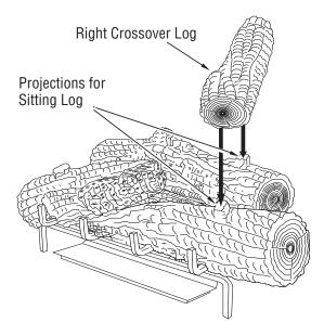
Figure 38 - Installing Right Crossover Log
