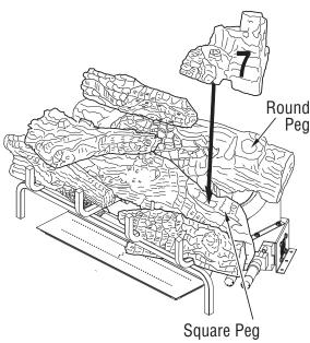
Figure 28 - Installing Log # 7
