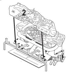
Figure 23 - Installing Log # 2
