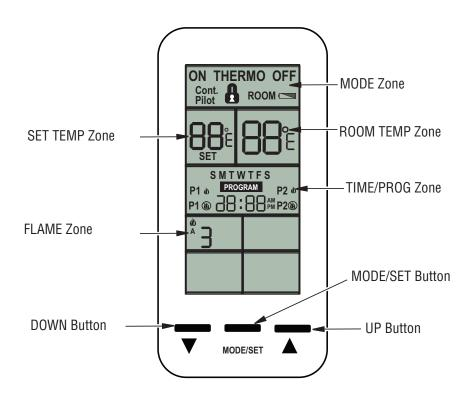
Figure 52 - Touch-Screen LCD and Button Layout
