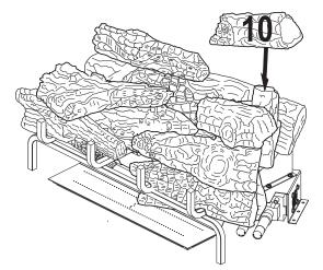
Figure 31 - Installing Log # 10
