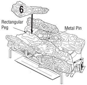
Figure 27 - Installing Log # 6
